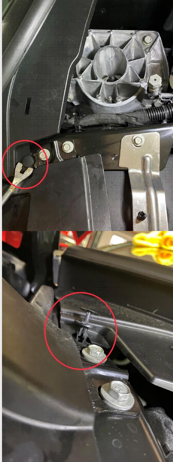
7. Slide the passenger side strut cover into place by angling the cover towards the
