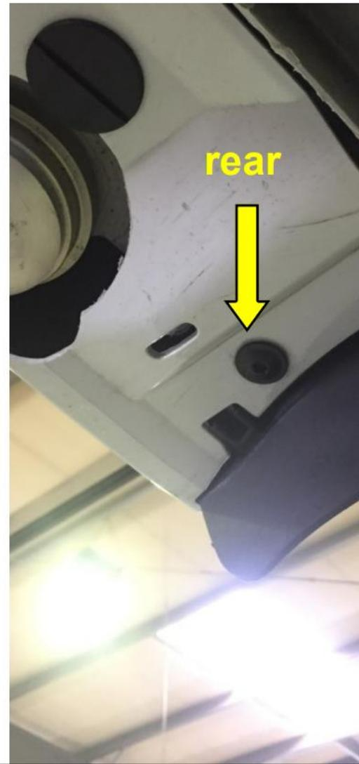
9. Remove all large plastic clips at the bottom of the door sill by twisting them (90°).
