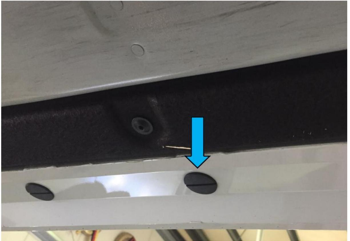
10. On the areas marked red, the door sill is fixed in holding strips by means of snap-in lugs. Carefully pull the door sill out of the retaining tabs.
