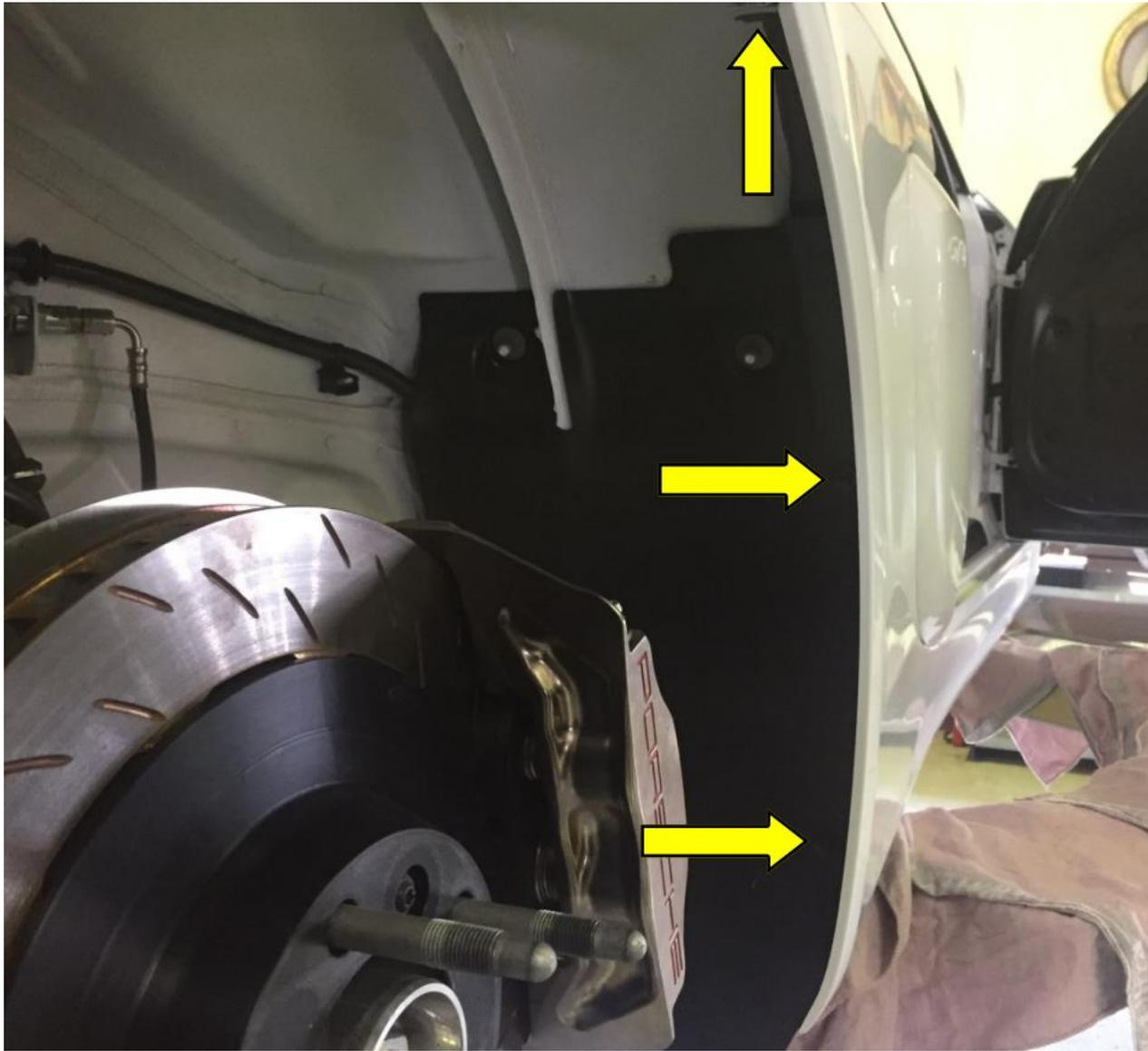
8. The door sill is fastened to the underside of the vehicle in the front and rear area with a screw. Remove them.
