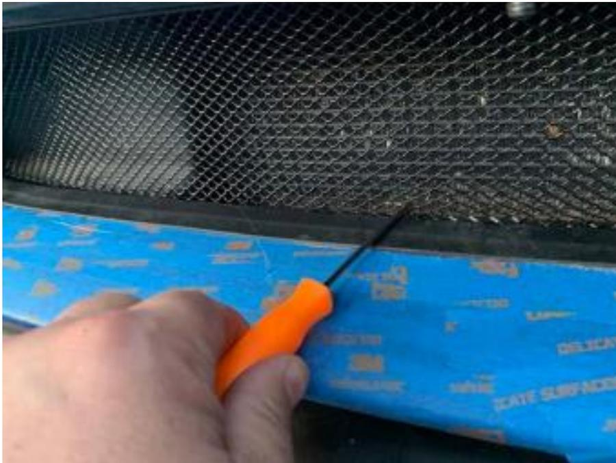
7. Now on to the easy ones!! If you made it this far, it is all downhill from here! Both sides install the same, so we will only demonstrate one side. To position the cable ties appropriately for your vehicle, you will need to install one side, mark where the cable ties go (I usually just place the cable tie through the hole noting with way they need to enter the hole next to it so it aligns with the lower vertical slats under the horizontal rib).
