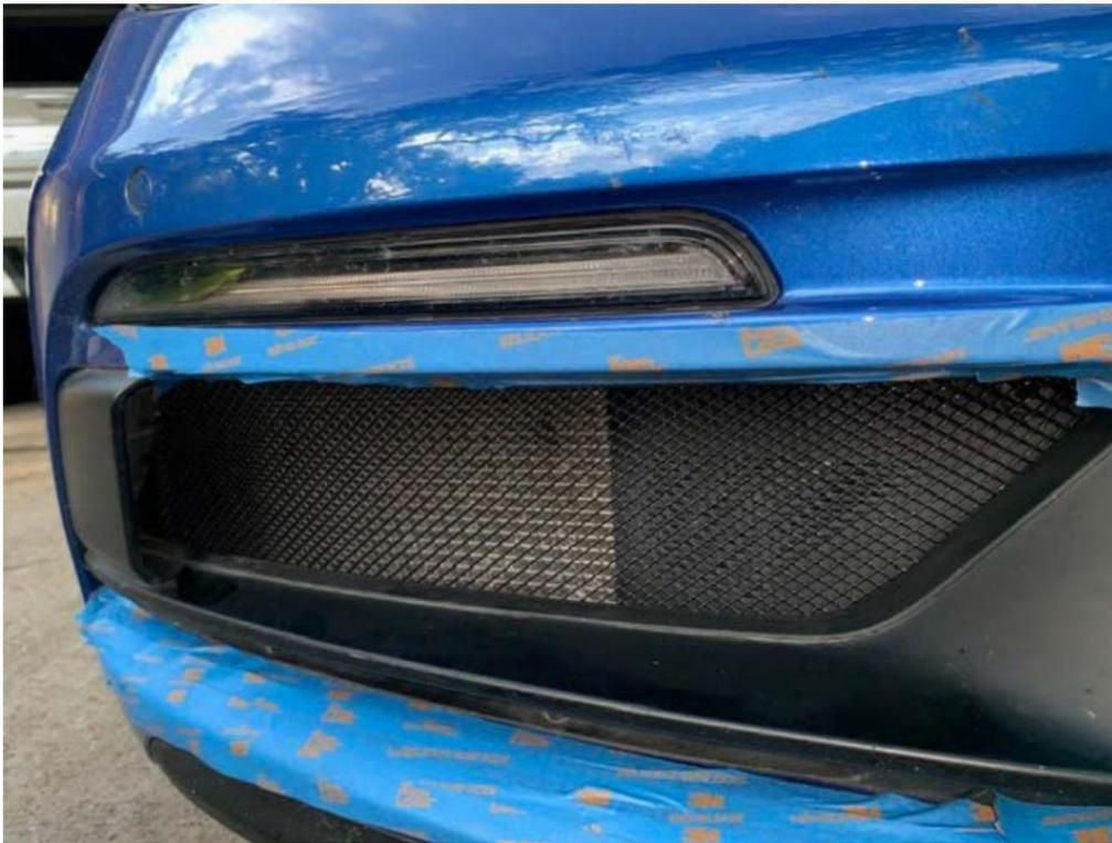
9. Using screwdriver/hooks, slide screen from left to right into groove (shown in the first photo is the right grille, but same concept, slide into the space between the outer bumper cover and the inner air dam):
