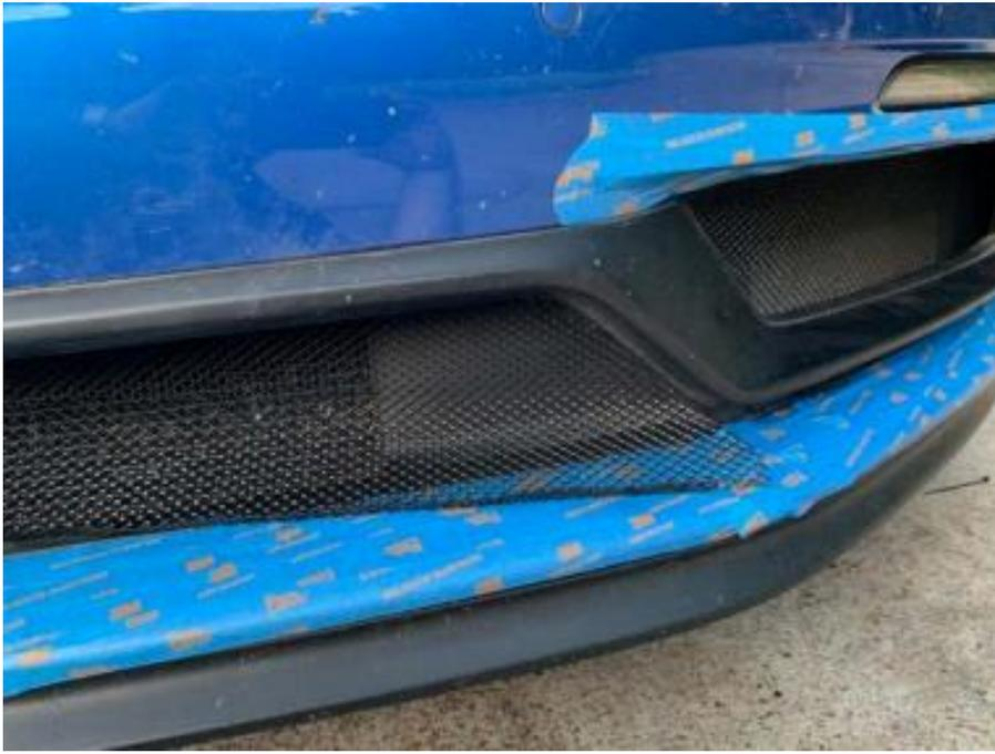
5. Once installed it will be far back in the cavity, work it forward and work the upper part of the grille in between the bumper and the ducting while working the lower lip under the bumper lip.
