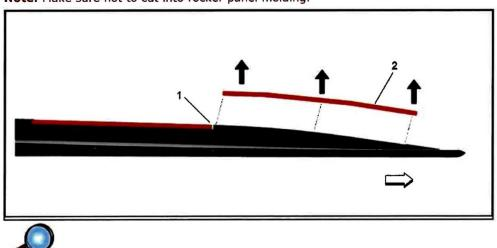
4. Remove the section of adhesive tape (2) from the rocker panel molding at the previous cut line (1).
