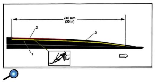
Note: Make sure to confirm adhesive tape area on rocker molding prior to applying primer and urethane. Refer to **Rocker Panel Adhesive Tape Modification** at the beginning of these instructions.
