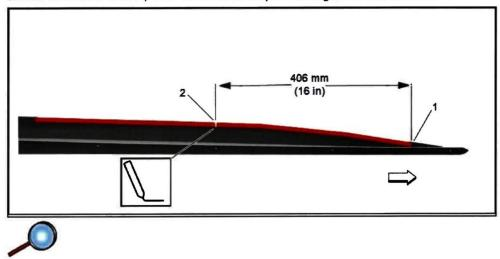
2. From the end of adhesive tape (1) at the front of rocker panel molding, measure 406mm (16 in) and mark a line (2) on adhesive tape liner.
