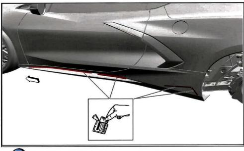
15. Note the area of attachment tape contact to rocker panel. Clean the area with the solvent wipe.
