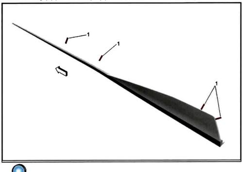
Peel back and expose tape liners (1) on the outside of rocker panel molding, do not fully remove liners.
