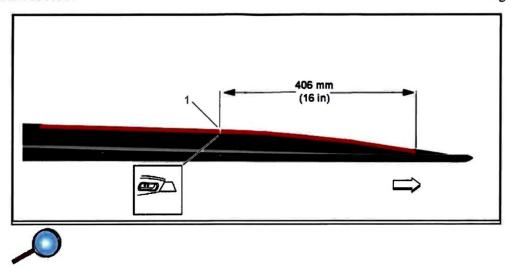
**Note:** Prior to cutting adhesive tape, peel back adhesive liner from front of rocker panel molding to the previously marked line (1). Leave adhesive liner long at cut to allow pull tab for install.
