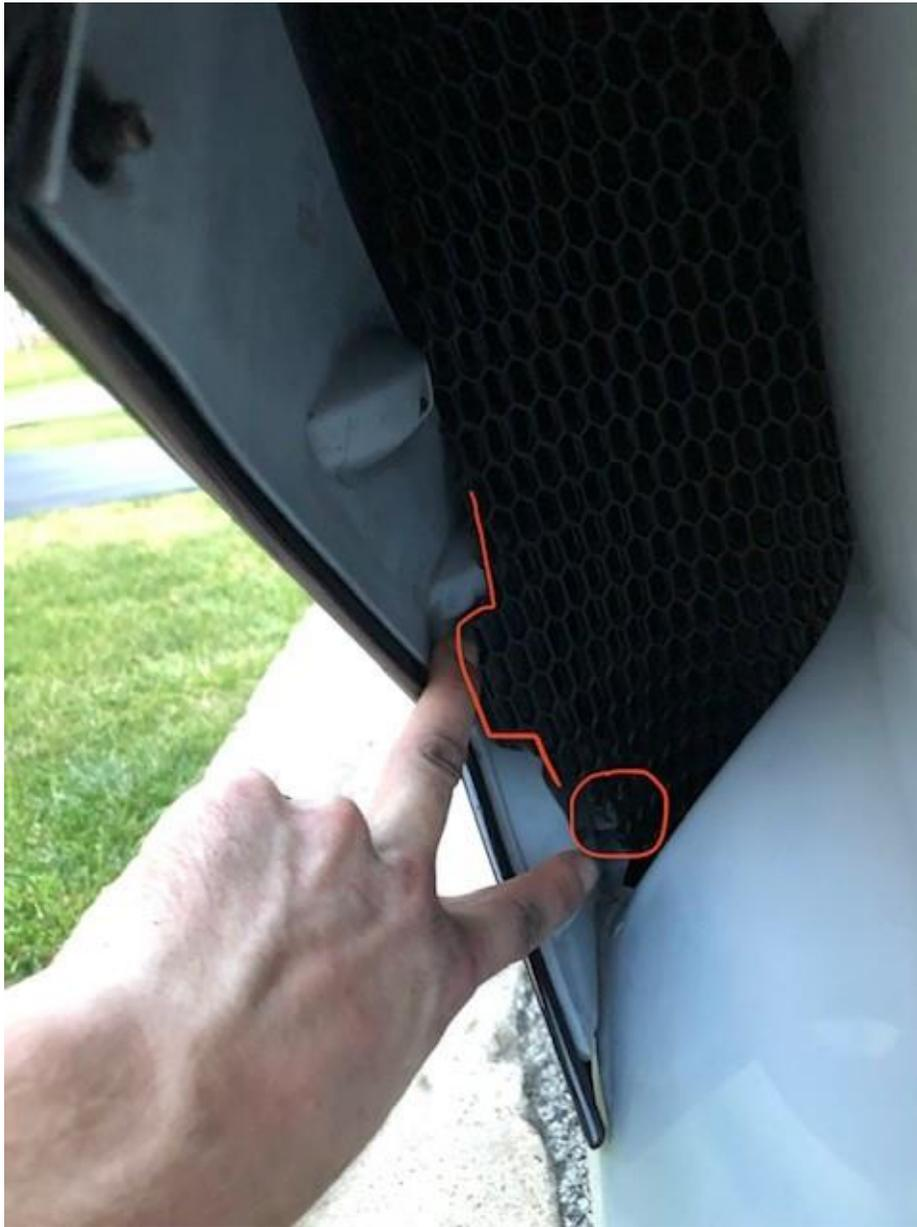
The circle shows where the side intake mount bolt now resides. All hidden and pretty now! Also this shows where the rectangle protrusion contacts the outer grille body part. Once in position you are done! Rinse and repeat! Contact us with any questions, we are here to help!!
