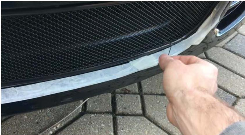
5. Press down all along the trim to ensure adhesion. Hold the trim to the emblem tape for a couple seconds to ensure good adhesion.
