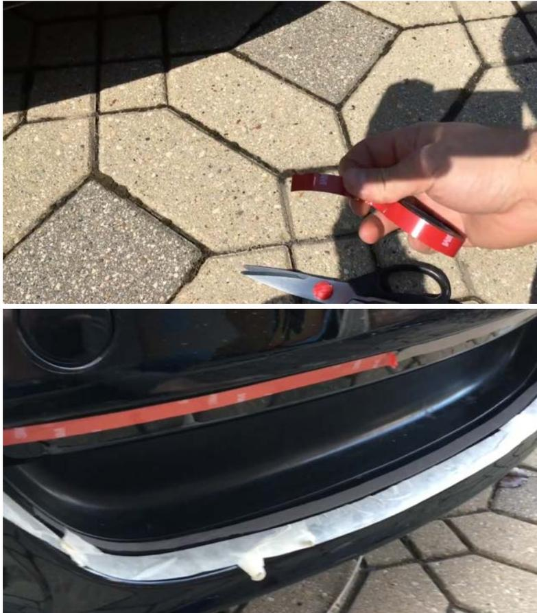
4. Once the tape is applied, position grill into tape. It may require pushing or pulling on the bumper cover to fit. You can use an allen wrench to pull the grill into position to hide the emblem tape as much as possible.
