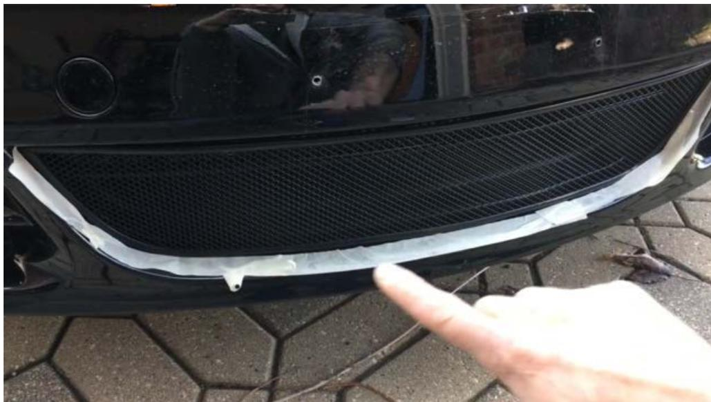
3. Remove the grill and prepare the 3M emblem and molding tape. You may want to split the molding tape to get a thinner profile. Cut the 3M tape down the middle and place just to the inside of the painters' tape line you just made. Peel back the protective backing.
