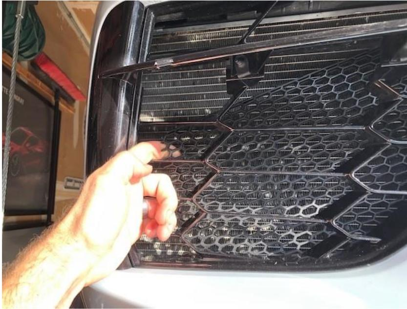
6. As the grill is fed through, it should be guided up towards the top of the radiator cavity. Align the grille and insert the cable ties where necessary, do not tighten. Insert all cable ties that you desire. You can see in the photo the locations we chose (the red circles on the bumper indicate cable ties behind, one for the brake duct grille and one to tie the brake duct grille to the large radiator grille). Loosely secure.
