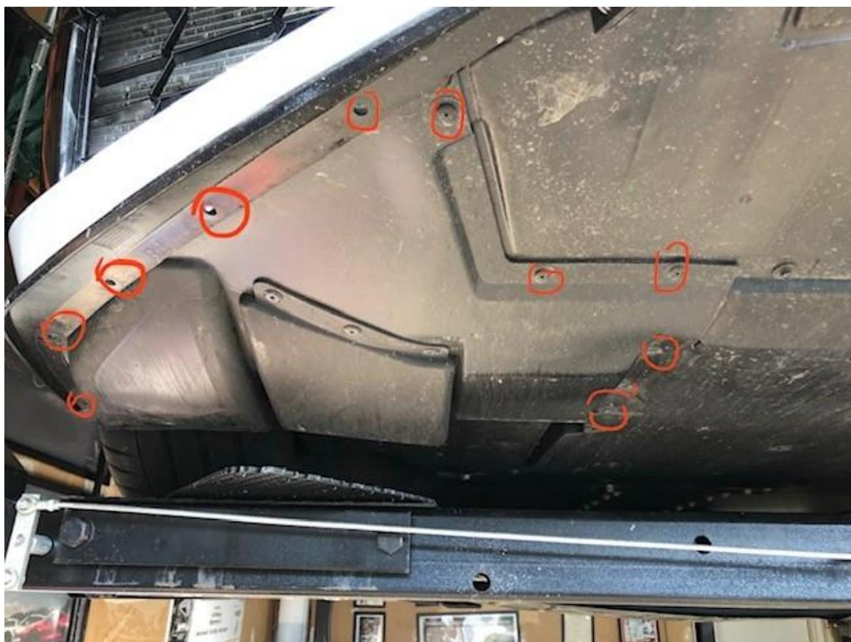
3. Remove the approximately 10 torx screws and 9/32 or 7mm bolts on each of the side panels and the panels drop down giving you room to fit the grille behind the stock fascia. The center panel does not need to be unfastened.
