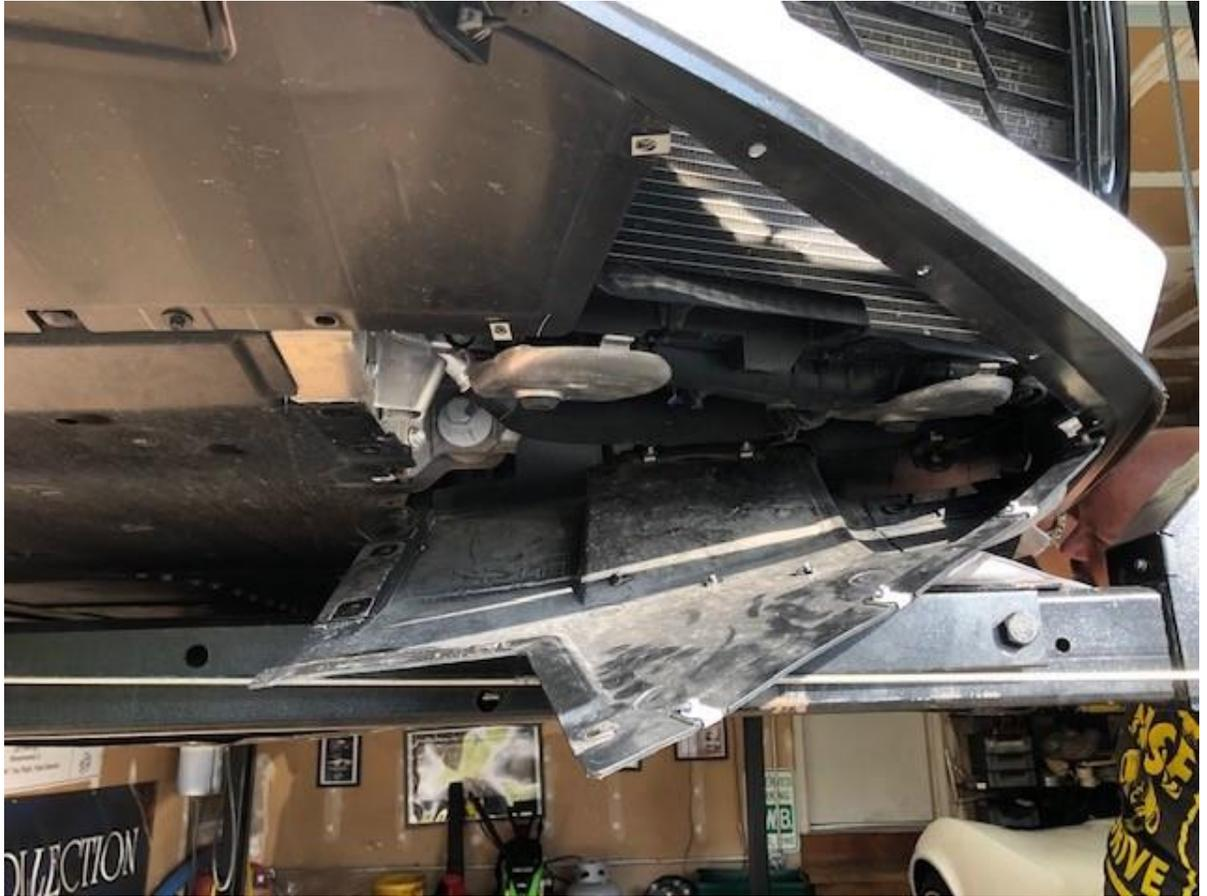
4. If you have the brake duct grille, this is the time to insert it into position. The brake duct grille inserts tightly into the brake duct area, the grill will slip about 1/2 inch behind the center section of the bumper. Don't worry about alignment, we will final align after the large radiator grille is in place.
